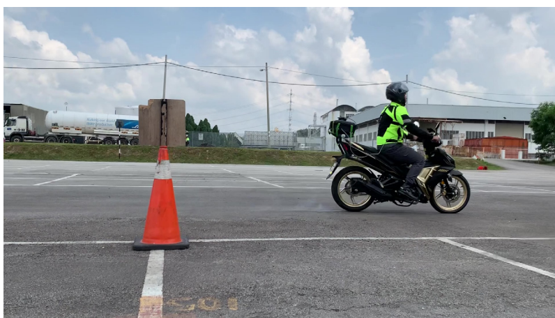
FIGURE 3. Experiment setup showing rider applying the brake at the start of traffic cones.
