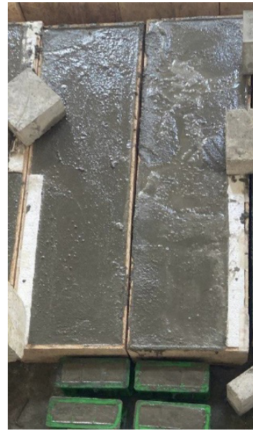
FIGURE 1. Casting of Wall Samples
