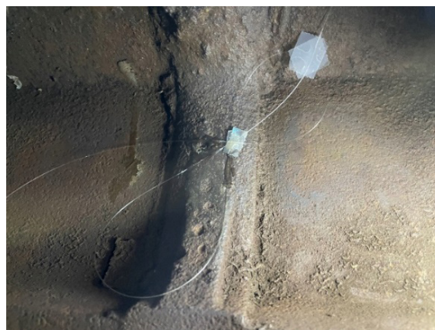
FIGURE 3. FBG sensors are installed on the web section of the rail
