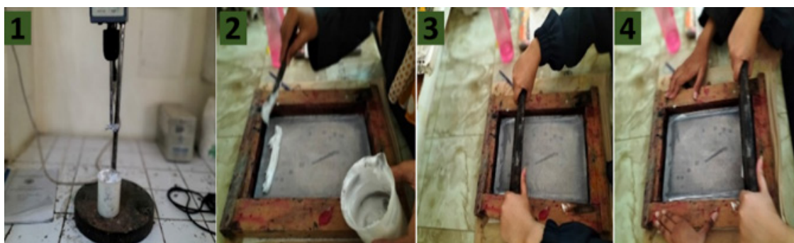
FIGURE 1. Screen printing of silica NPs on cotton fabric preparation 1 , incorporation 2 on mesh, application 3 of coating paste on cotton fabric and dragging and squeegee of fabric for uniform application 4
