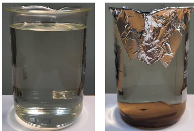
FIGURE 3. Sealed untreated mineral oil with pressboard samples
