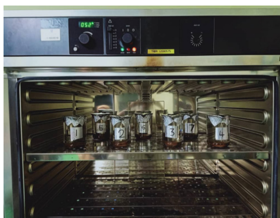
FIGURE 4. Sealed untreated mineral oil and pressboard samples in hot oven
