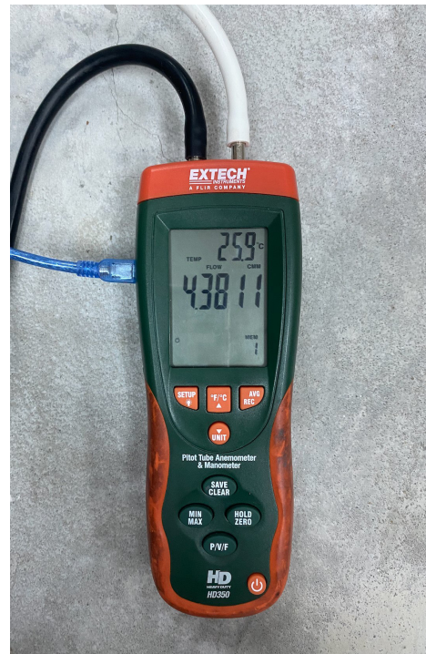
FIGURE 9. Pitot tube anemometer used to measure flow rate
