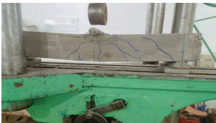
FIGURE 5. Crack pattern at failure of set H
