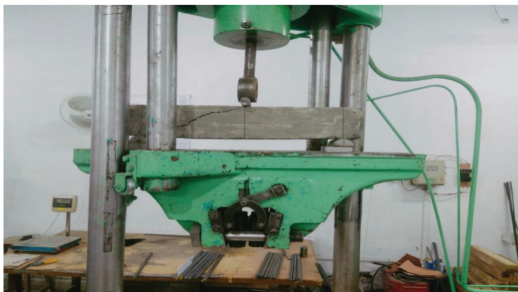
FIGURE 4. Crack pattern at failure of set A
