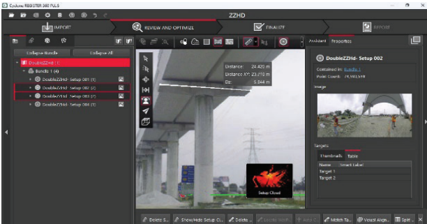
FIGURE 13. Point cloud features measurements
