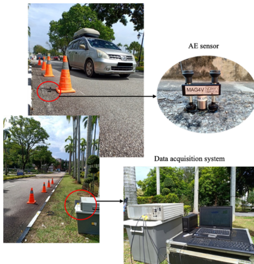
FIGURE 3. AE real-time monitoring test setup
