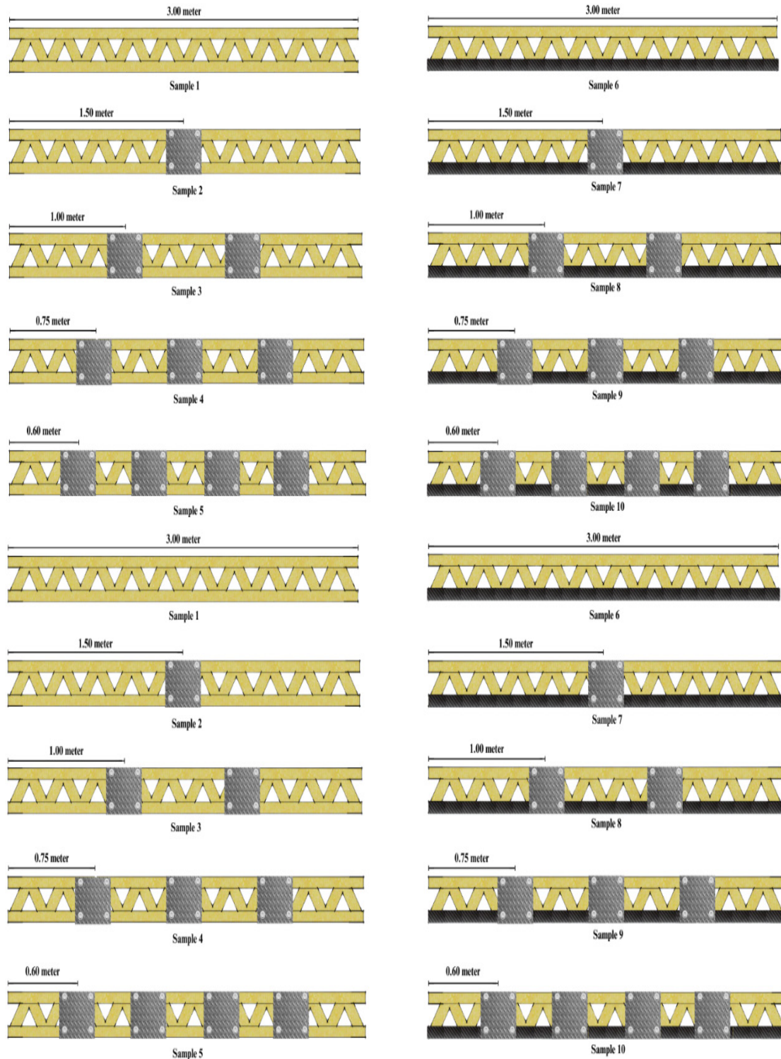
FIGURE 2. Sample without reinforcement (top) and with reinforcement (bottom)
