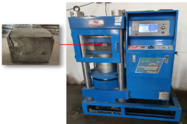
FIGURE 3. The set up of the compressive strength testing of the mortar cube
