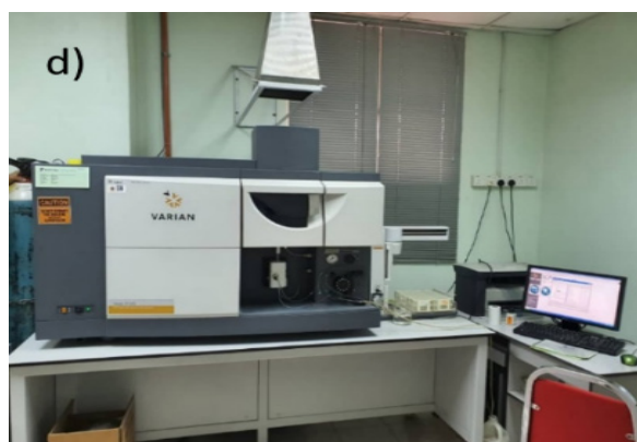
FIGURE 4. Heavy metal elements measurement done by ICP - OES machine
