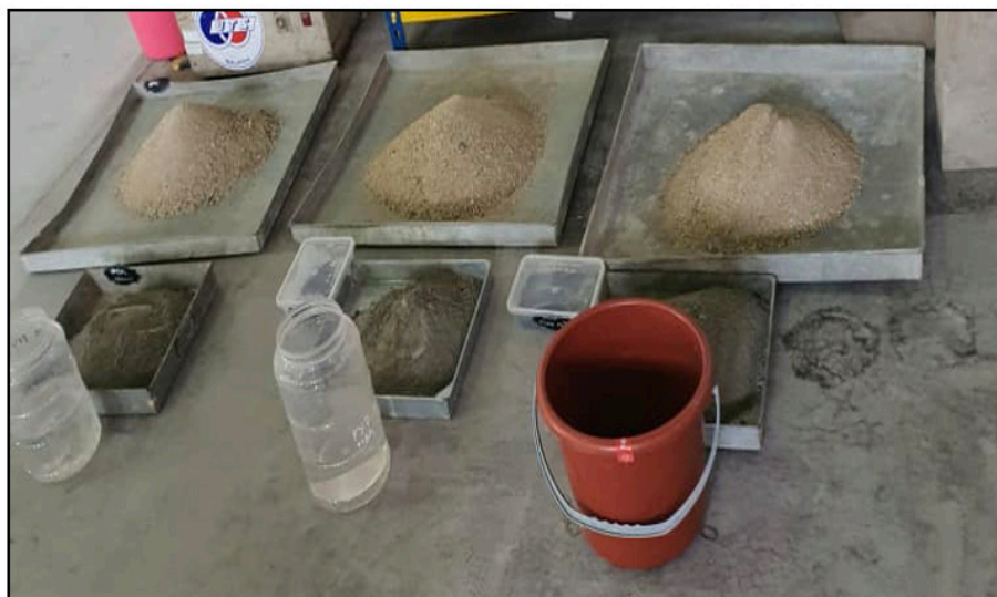
FIGURE 2. Batching of materials according to mortar proportion
