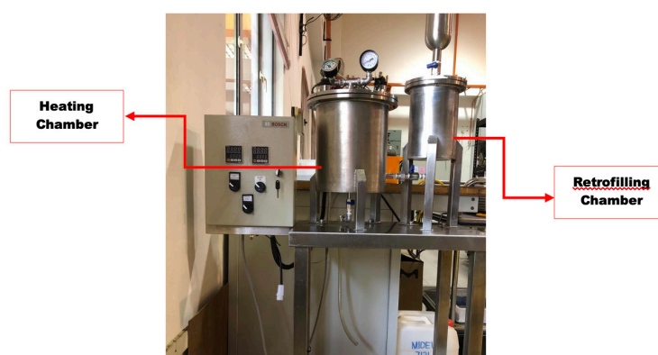
FIGURE 1. Experimental setup used for accelerated thermal ageing
