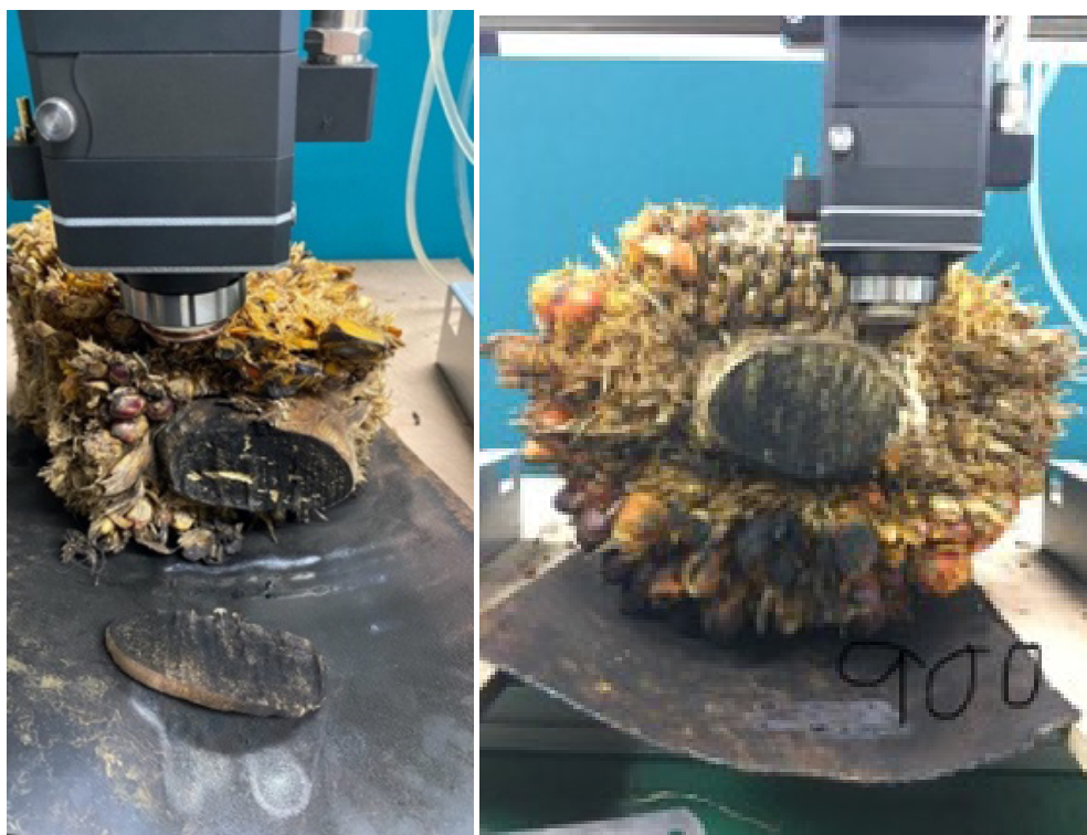
FIGURE 6. Laser cutting test on FFB stalk sample
