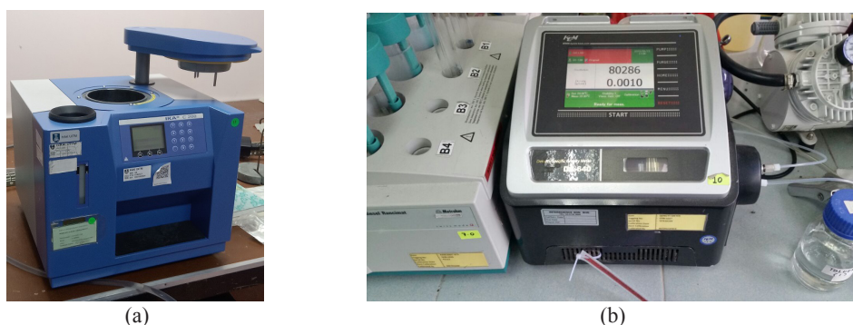
FIGURE 3. Properties Tests, (a) Bomb calorimeter, and (b) Digital Density Meter
