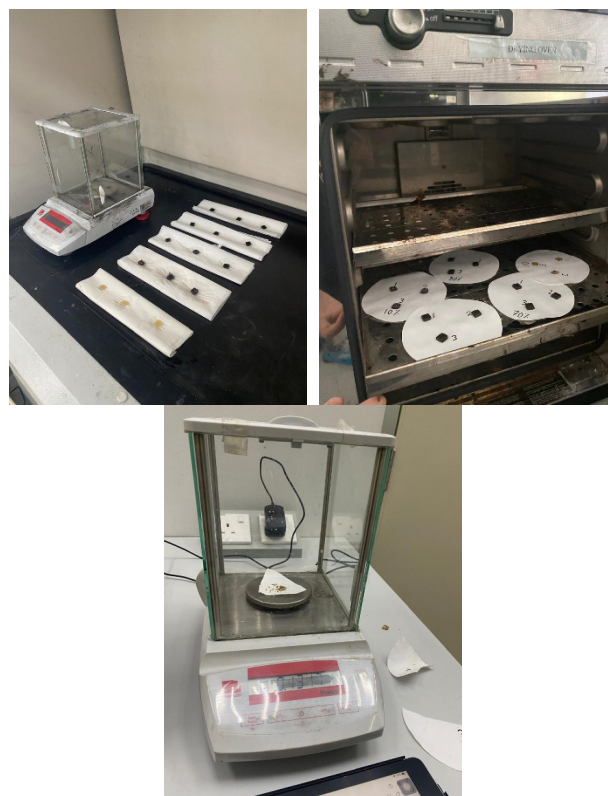
FIGURE 6. Moisture content procedure of weighting before oven dry and weighting after the oven dry.
