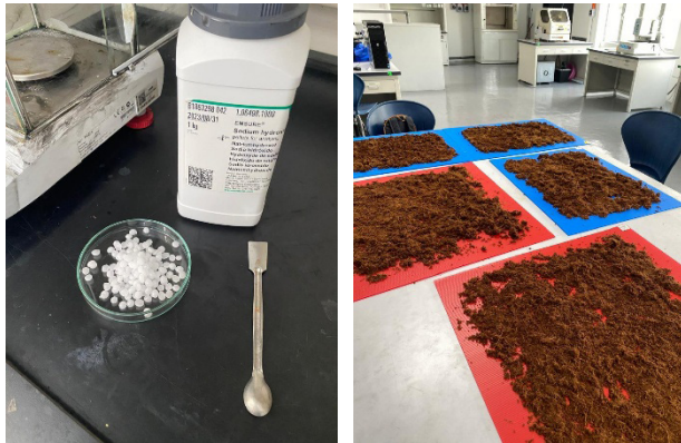
FIGURE 3. Process of alkaline treatment on coconut husk fibre.
