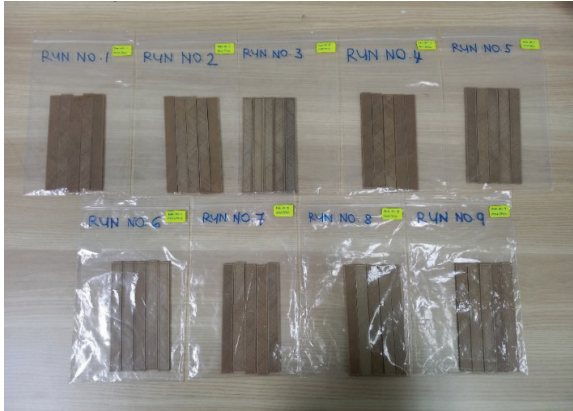
FIGURE 4. The samples specimen of PALF/PLA (ASTM D790)
