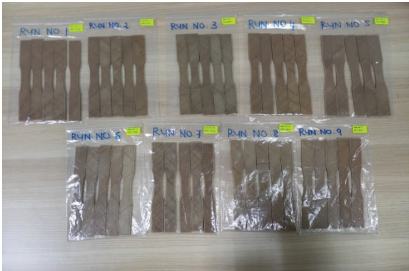
FIGURE 3. The sample specimen of PALF/PLA (ASTM D638 Type I)
