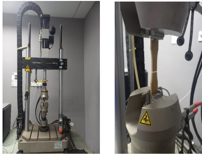
FIGURE 5. The Instron 8872 UTM Machine for Tensile Testing
