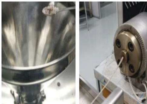
FIGURE 4. Filament produced from the extrusion process
