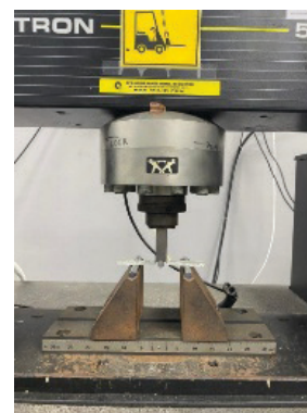
FIGURE 8. The flexural testing by pin Instron Universal Testing Machine (UTM)
