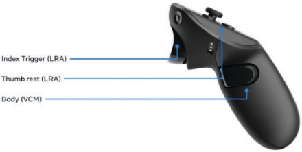
FIGURE 19. Haptic feedback system on Meta Quest Touch Controller
