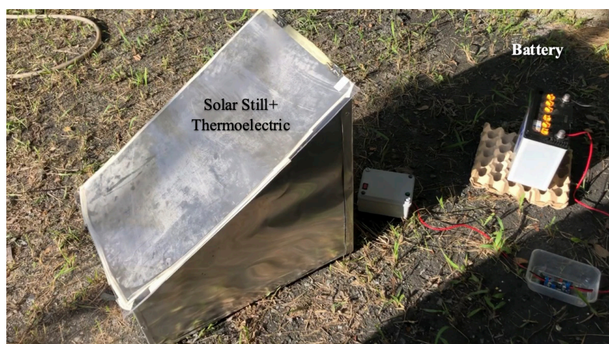
FIGURE 3. Solar Still with Thermoelectric System
