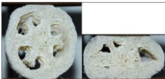
FIGURE 14. Luffa sponge under lateral loading (An et al. 2015)
