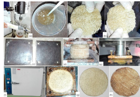
FIGURE 11. Explains (a) Chitosan gel (b) Luffa layers impregnated with chitosan (c) Two covered rigid plates (d) Placing the impregnated Luffa-chitosan between two platens applying quasi-static load on the impregnated layers (f) Processing the panel in an oven (g) Panel of Luffa-chitosan (h) Panel of glass-chitosan (Goudarzi et al. 2022).
