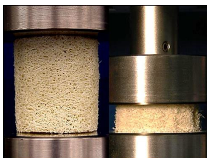
FIGURE 7. Luffa sponge under axial compression loading (Shen et al. 2014)
