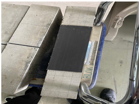
FIGURE 4. The 250mm x 500mm CFRP plate
