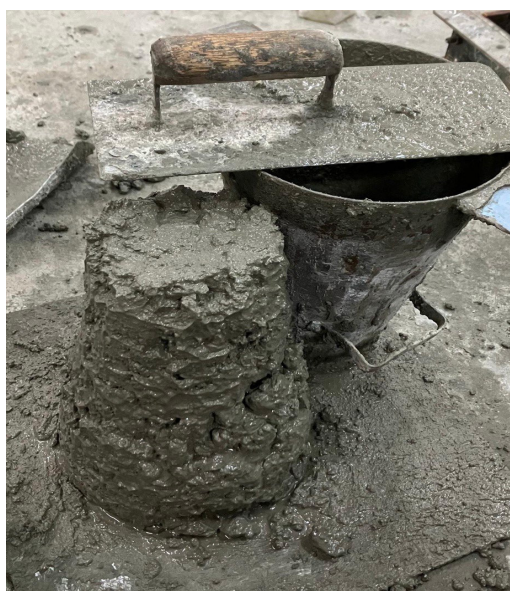
FIGURE 6. The slump test
