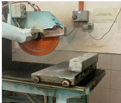
FIGURE 3. Notch cutting process
