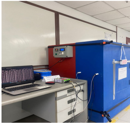
FIGURE 1. Hot box testing setup
