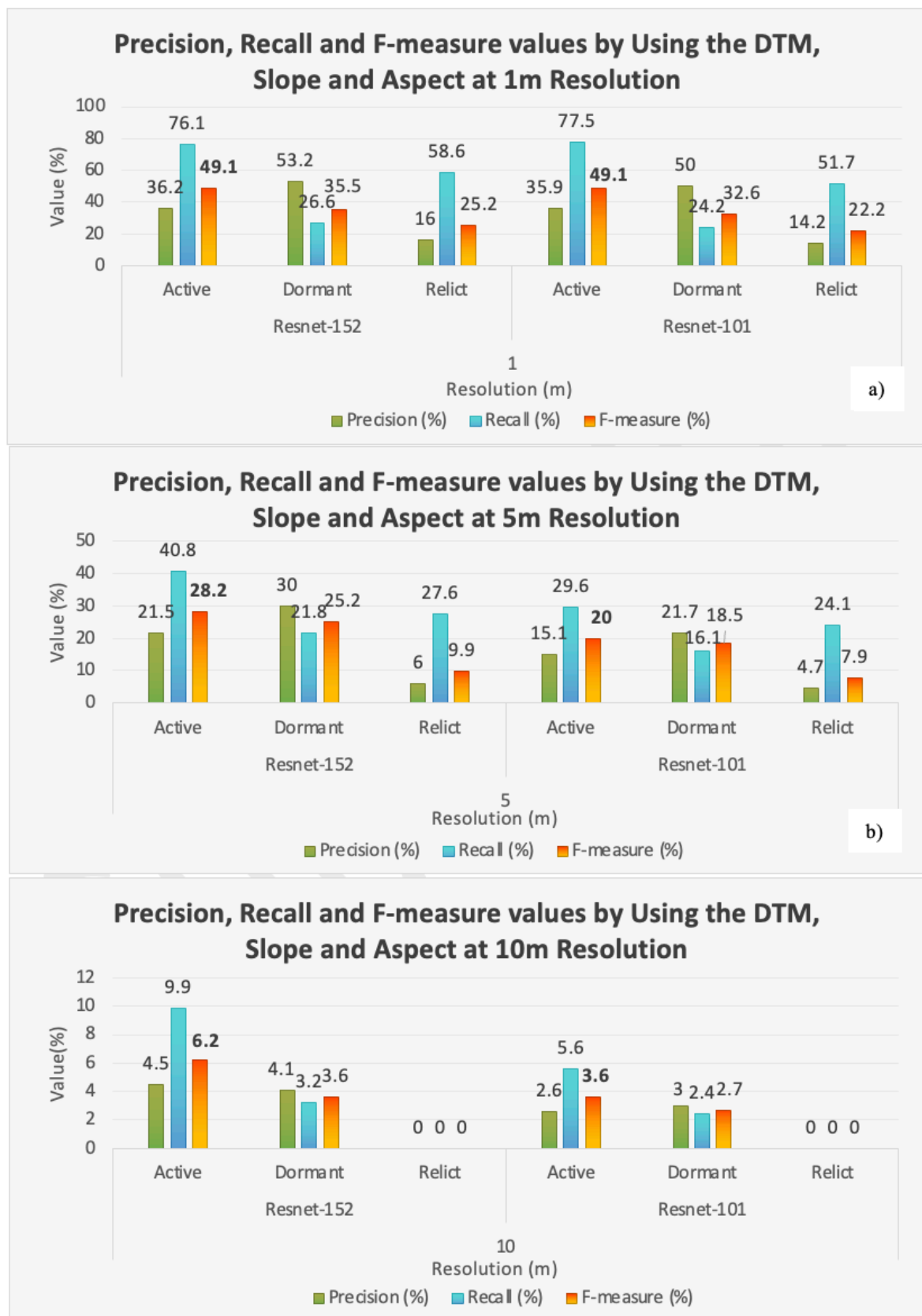
FIGURE 12. Precision, Recall and F-measure values obtained for landslide detection a) at 1 m resolution, a) at 5 m resolution and a) at 10 m resolution by using the DTM, slope, and aspect input parameters
