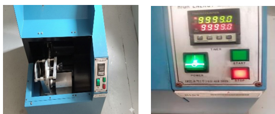
FIGURE 4. High-energy ball milling machine for powder mixing process and powder compaction
