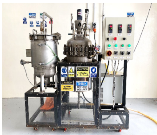
FIGURE 3. Experimental setup of the 70 L SWE system and its main components
