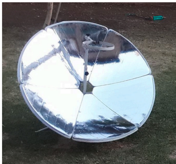
FIGURE 4. A photograph of the parabolic dish solar cooker used in the cooking tests
