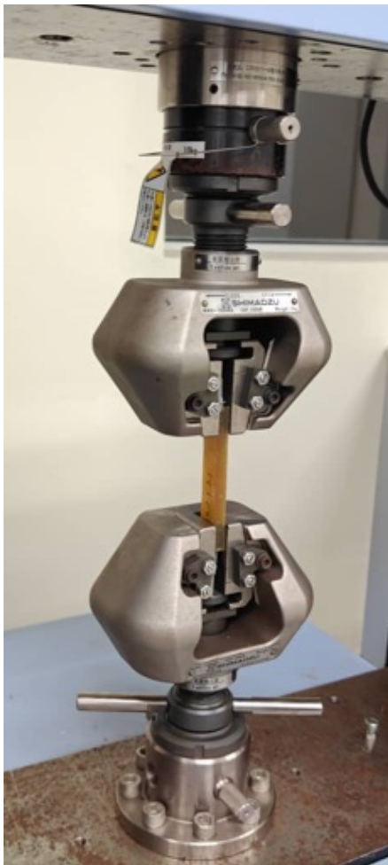
FIGURE 4. Tensile Strength Test Experimental Settings
