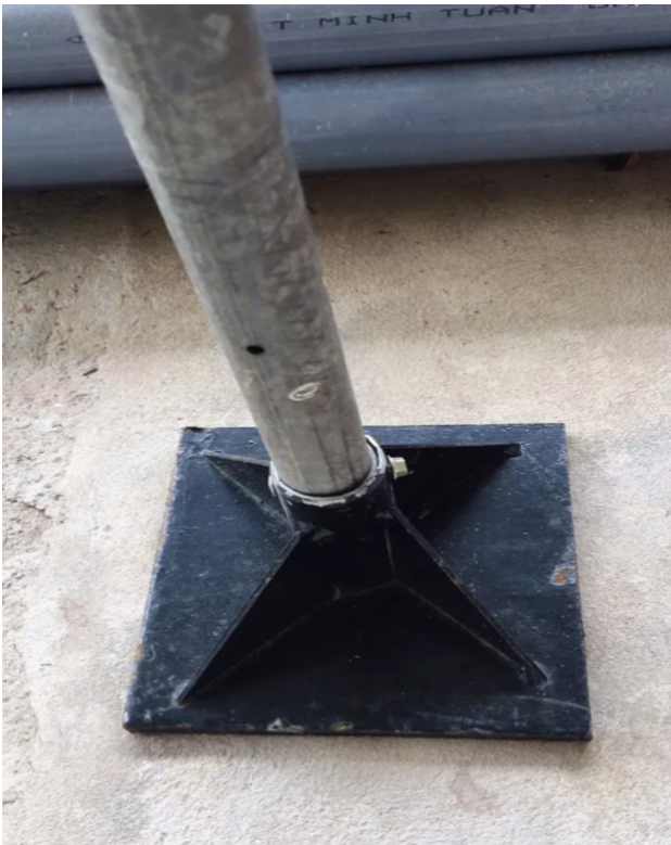
FIGURE 8. Hand compactor for manual compaction
