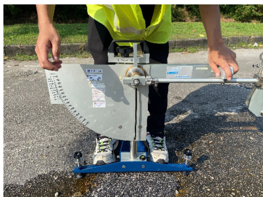
FIGURE 11. Skid Resistance Test Using British Pendulum Tester
