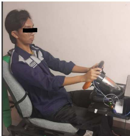
FIGURE 5. Complete experimental setup showing simulator, HR sensor system, and auditory warning mechanism.
