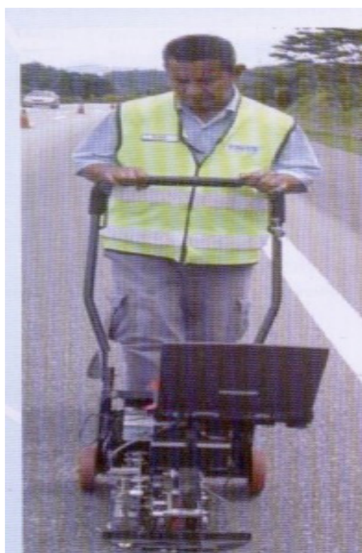
FIGURE 2. Walking Profiler roughness measurement
