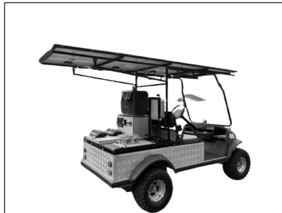
FIGURE 5. Example of a Mobile Solar Charging System
