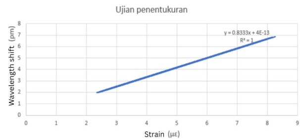
FIGURE 9. Strain test results for determining the sensitivity of the FBG sensor
