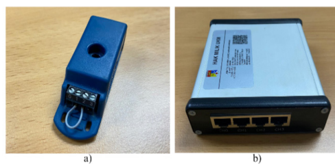
FIGURE 4. a) NI-9945 module b) Data Acquisition (DAQ) system
