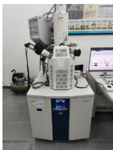
FIGURE 9. Scanning Electron Microscope HITACHI - SU5000
