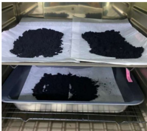
FIGURE 5. Waste tyre rubber in the oven
