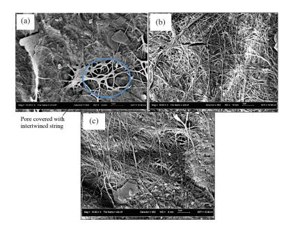
FIGURE 1. SEM image for (a) oven drying, (b) tray drying and (c) freeze drying
