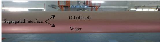
FIGURE 2. Stratified flow pattern (ST)
