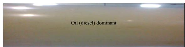
FIGURE 4. Water-in-oil dispersion flow pattern ( $D_{w/o}$ )
