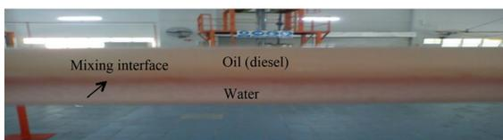
FIGURE 3. Stratified with mixing interface flow pattern (ST &amp; MI)
