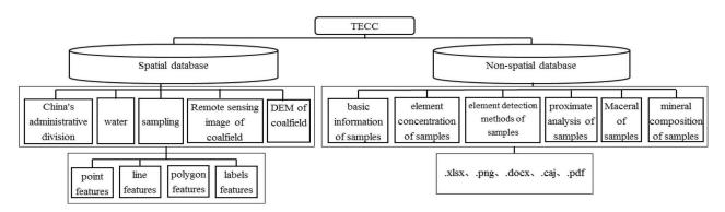
FIGURE 2. Structure of Data in TECC
