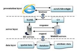
FIGURE 1. Structure diagram of B/S in TECC
