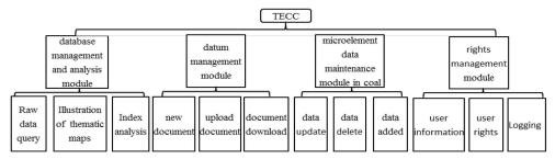
FIGURE 3. Functional structure of TECC
