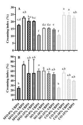
FIGURE 1. Creaming index of vegetable full-fat mayonnaises at room temperature (A), and hot temperature (B)
