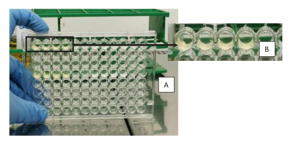
FIGURE 1. Samples were coated at the fixed area on the side of a well in a vertically positioned 96-well microtiter plate. B showing an enlarged image of A
