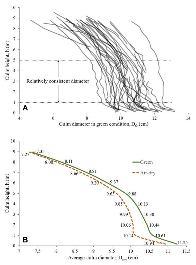
FIGURE 4. Culm height versus culm diameter. (A) Individual culm in green condition, and (B) Average values in green and air-dry conditions
