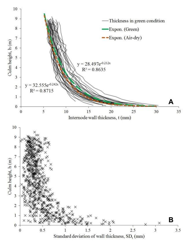
FIGURE 6. Graphs of internode wall thickness. (A) Culm height versus wall thickness, and (B) Culm height versus standard deviation in thickness measurements
