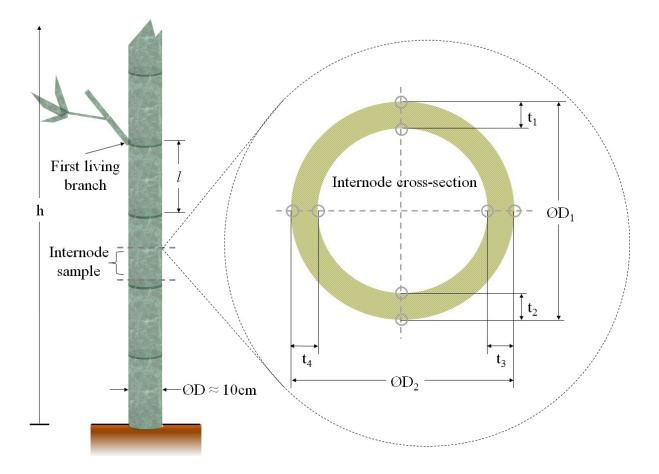
FIGURE 1. Measurements of the height of the first living branch, internode length, culm diameter and wall thickness
