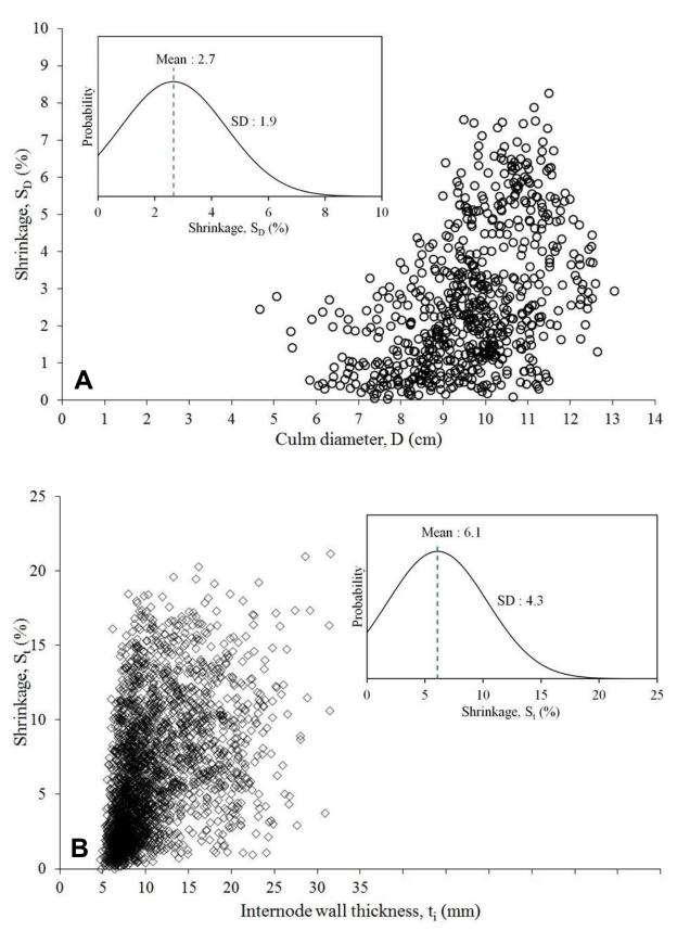
FIGURE 5. Percentage of shrinkage. (A) Culm diameter shrinkage, and (B) Internode wall thickness shrinkage
