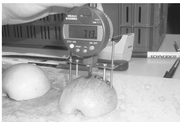
Figure 5-2. Radius of curvature meter using a Mitutoyo® height meter.
