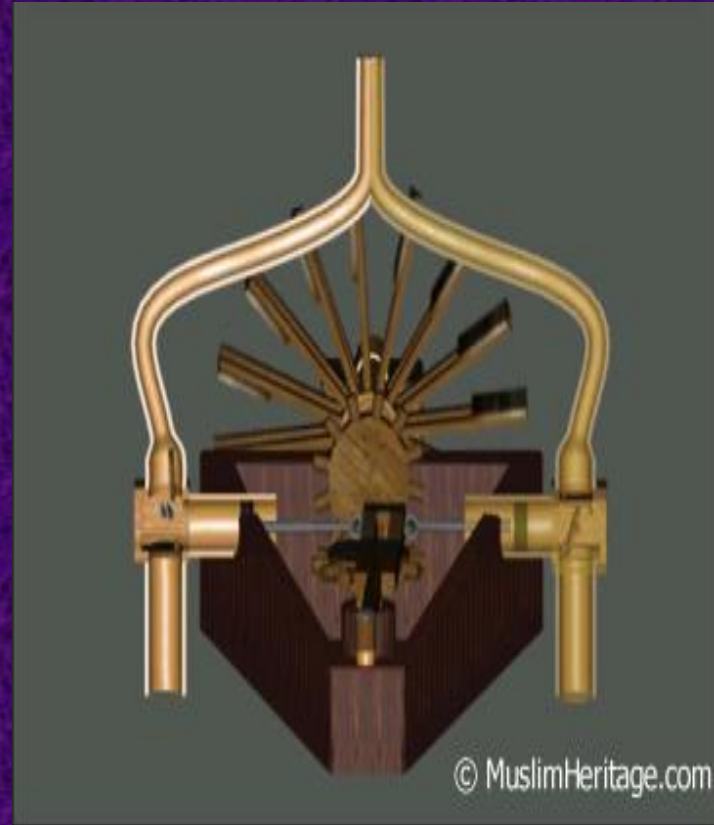
3D Image of the reciprocating pump with a water wheel as the drive source
