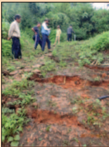
Figure 4: Cracks in the weathered leuco-granite rocks.
