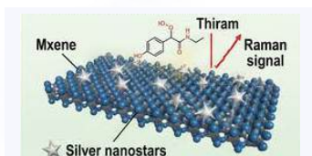
Two-dimensional titanium carbide (Mxene)/silver nanostars (AgNs) composite as SERS substrate for thiram pesticide detection
