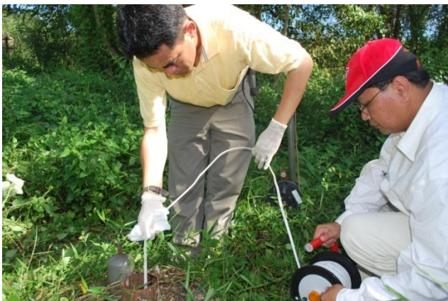
Measuring Groundwater Table Using Dip Meter
