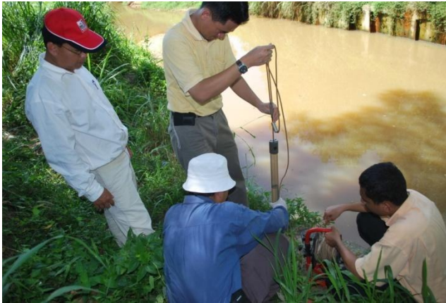
Collecting Groundwater Sample Using Bailer
