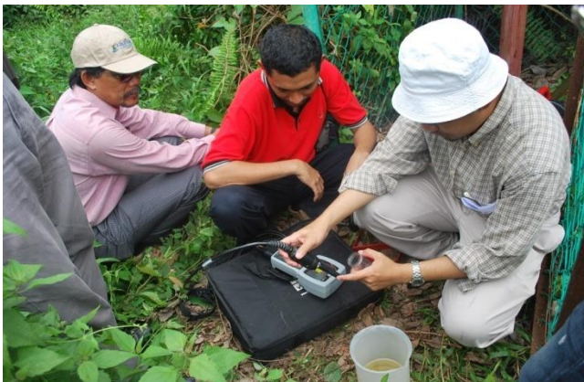
Measuring Water Insitu Parameters Using Multimeter Probe
